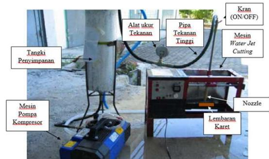
Gambar 3. Proses pengambilan data Mesin Water Jet Cutting
